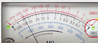
High resistance: Green LED lights up.
