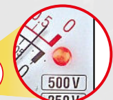
Low resistance: Red LED lights up.
