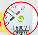
High resistance: Green LED lights up.
